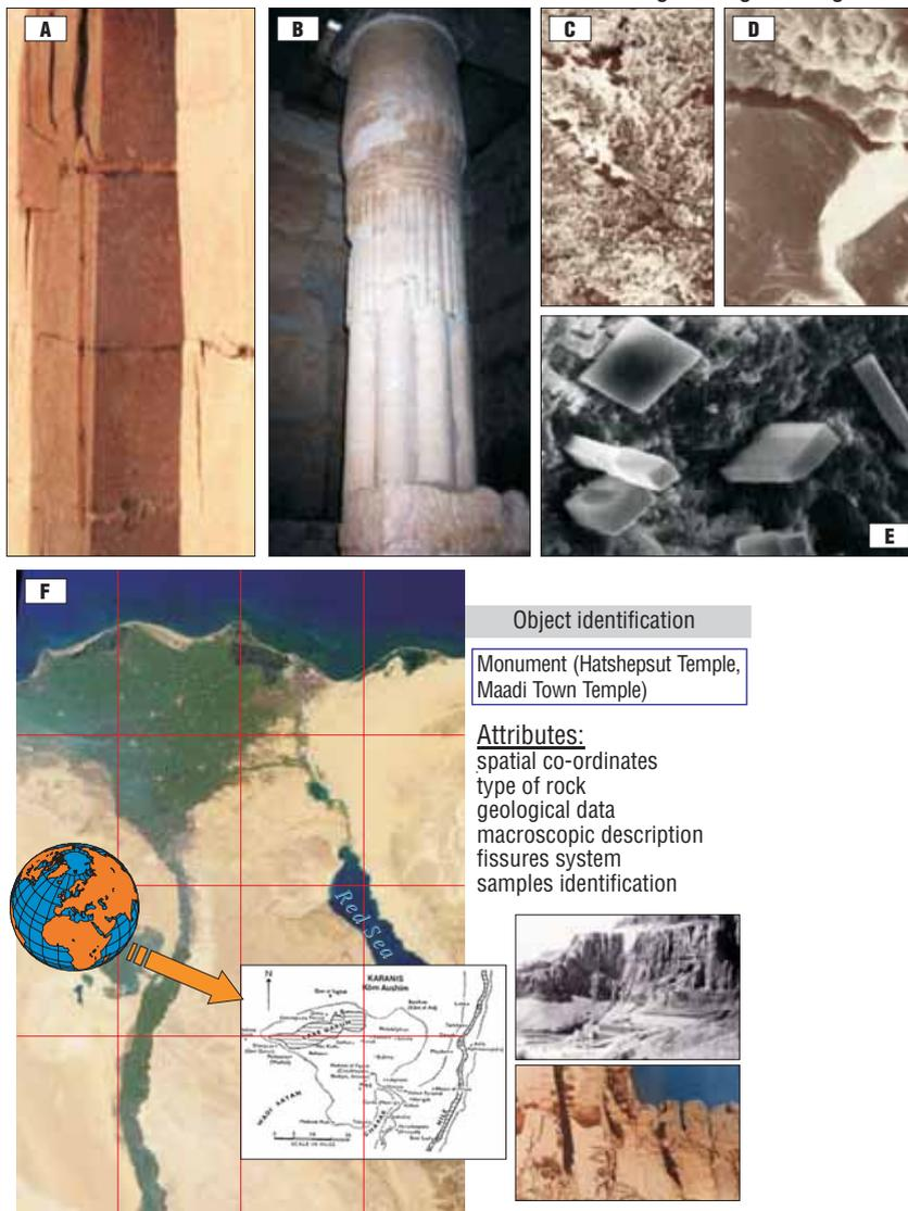
**Fig. 12.** Examples of the damages in the valuable stone elements of monumental objects: A — macroscale fracturing of the walls, B — efflorescence on pillars, C — closeup of the efflorescence (SEM), D — microfissure (SEM), E — salt crystallization (SEM), F — location of the described monuments
