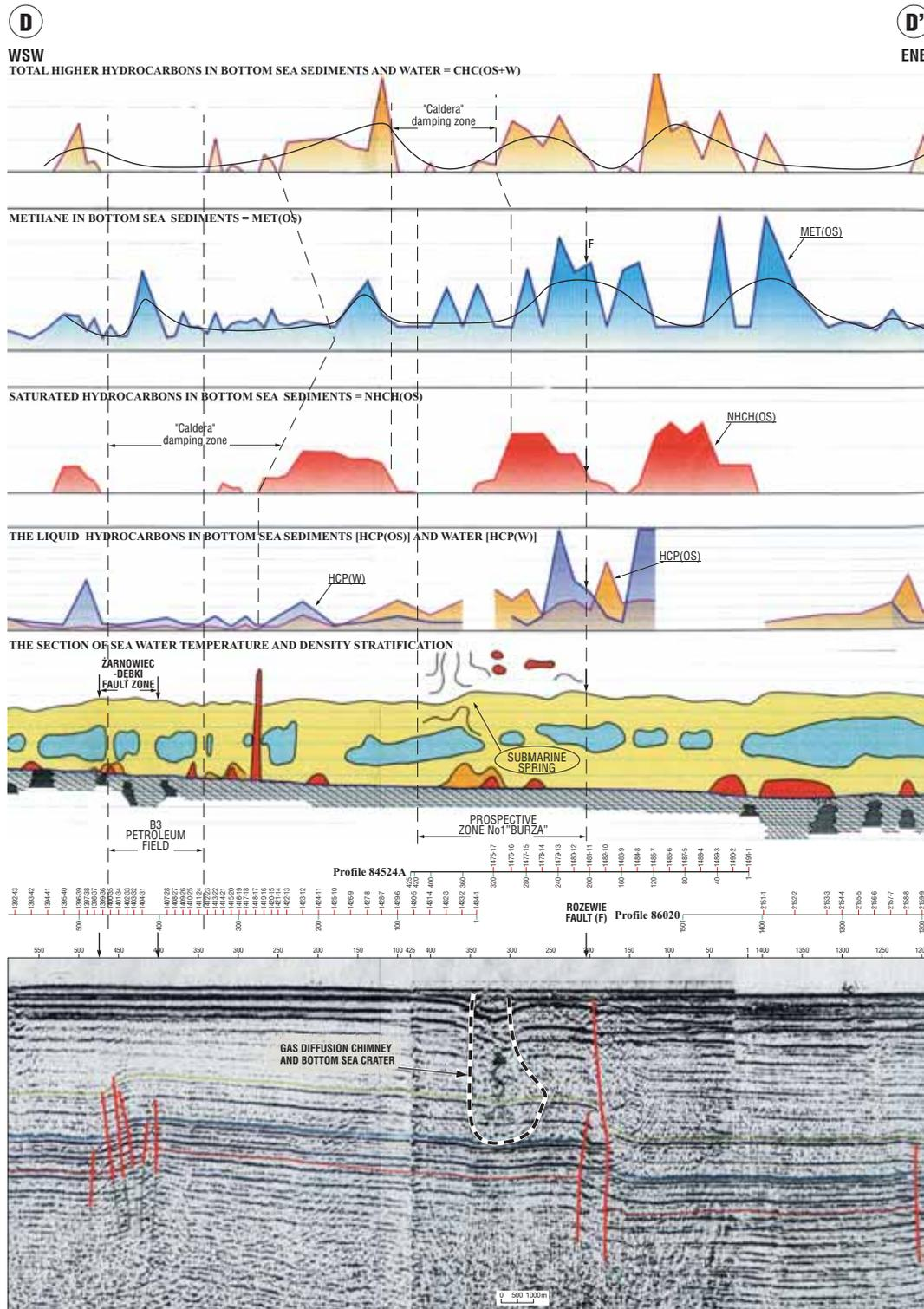
**Fig. 4.** Offshore geochemical-seismic profile D-D' (WSW-ENE) showing the location of B3 oilfield accumulated in a fault-confined anticline on the northern extension of the Żarnowiec-Dębki Fault zone (western ending of the profile) and the prospective zone "Burza" on the hanging wall of the meridional Rozewie Fault
