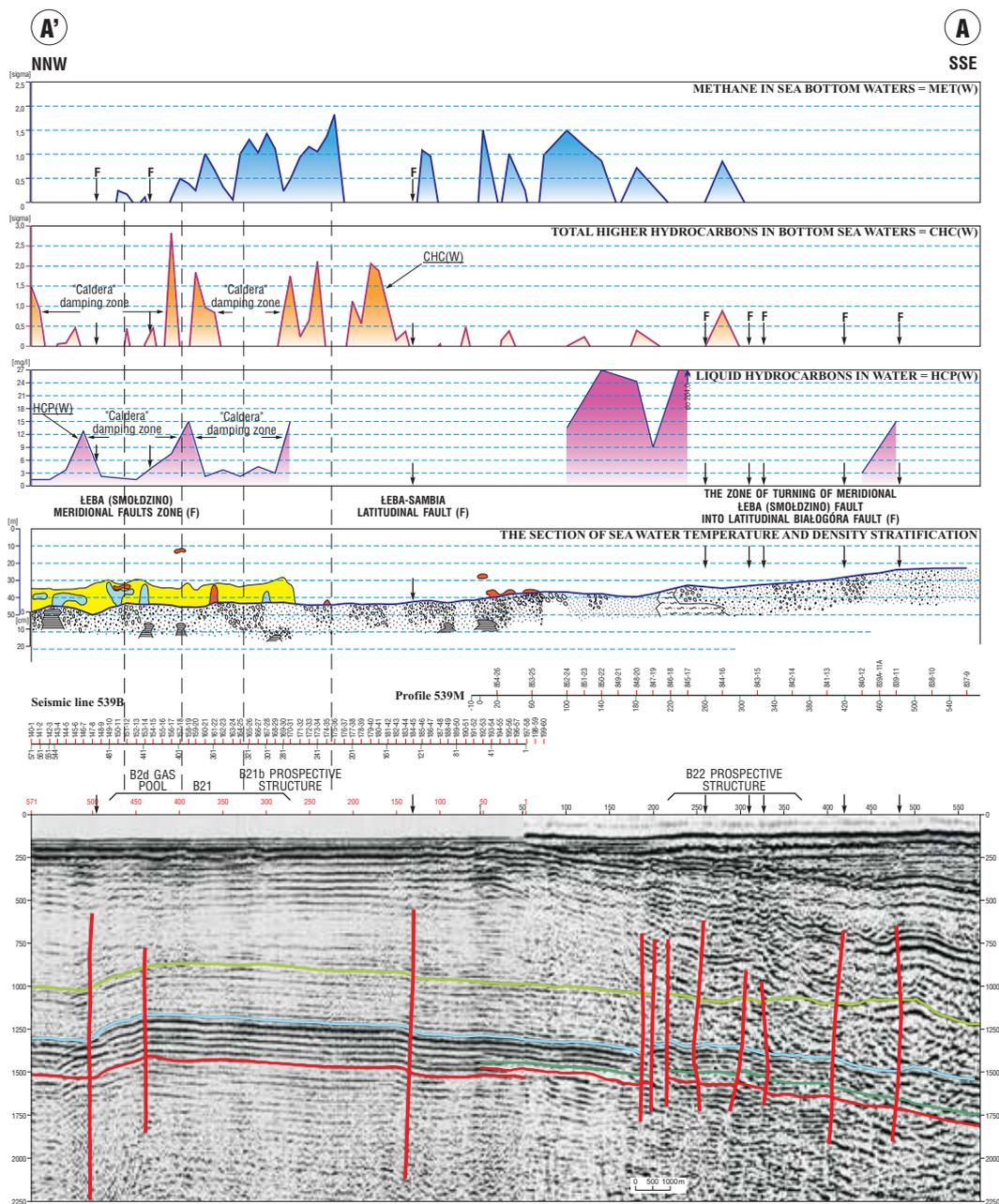
Fig. 2. Offshore geochemical-seismic profile A-A' (NNW–SSE) running from B21 gas-condensate deposit accumulated on hanging wall of the Smoldzino (Łeba) meridional fault to the tectonic crossing of the Smoldzino (Łeba) and the latitudinal Łeba–Sambia and Białogóra Fault
