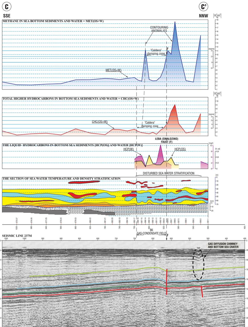
Fig. 3. Offshore geochemical-seismic profile C-C' (SSE–NNW) showing on its northern ending the location of B6 gas-condensate deposit accumulated on the hanging wall of the meridional Smoldzino (Leba) Fault
