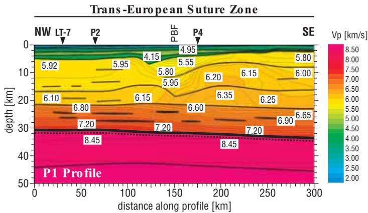
**Fig. 4.** The 2-D seismic velocity model along POLONAISE'97 profile P1 developed by forward ray-tracing technique (Jensen et al., 1999). The profile runs along the Trans-European Suture Zone (in the Polish Basin) almost parallelly to the edge of the East European Craton. The thick solid lines are layer boundaries and thin lines are isovelocity contours in km/s. Triangles refer to cross points with seismic profiles LT-7, P2 and P4. PBF — Poznań–Bydgoszcz Fault
