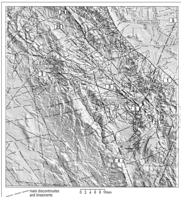
**Fig. 1.** The map of the main discontinuities and lineaments of the Kłodzko Valley superimposed at the DTM. For explanations of the labels of main discontinuities see text
