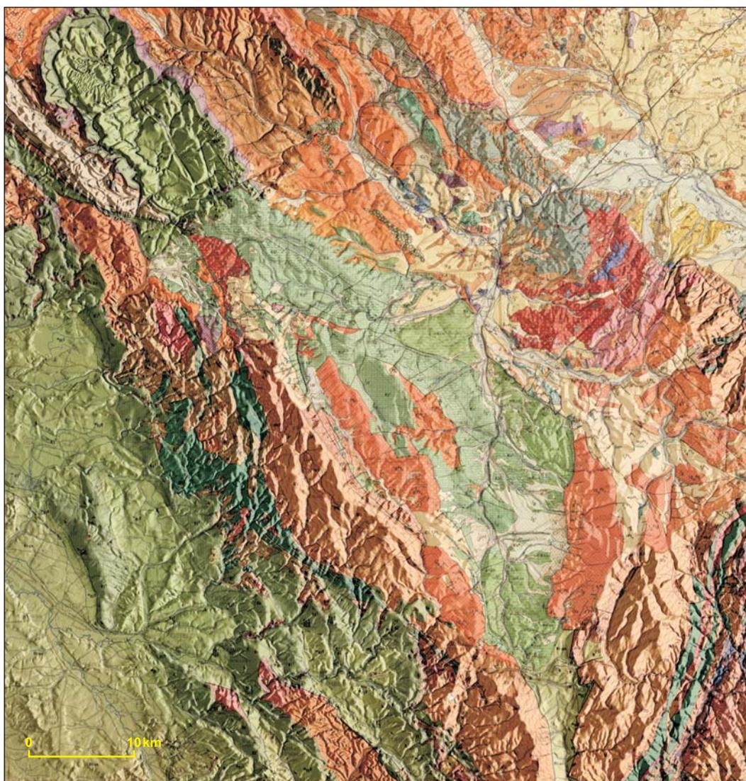
**Fig. 1.** An example of plastic visualization of a geological map. Geological map 1 : 200,000 (sheets Kłodzko and Nachod) superposed upon a shaded relief map, constructed on the basis of a digital elevation model DTED level 2
