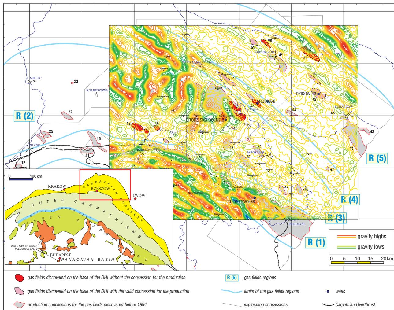
Fig. 1. Map of gravity residual anomalies superimposed on the map of hydrocarbon deposits and in the eastern part of the Polish Carpathian Foredeep (after Myśliwiec, 2004)
