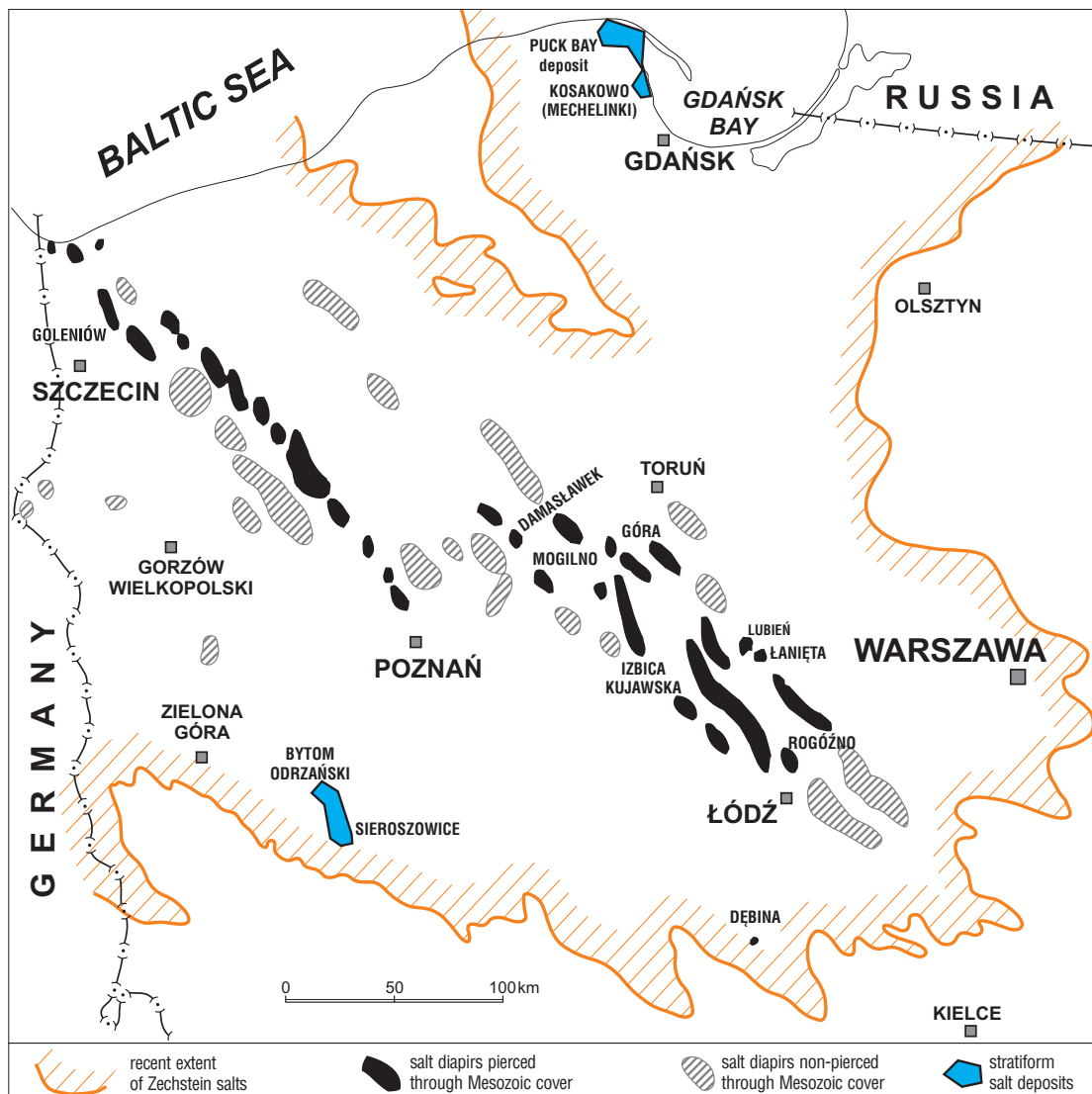
Fig. 2. Location of selected diapires of Upper Permian salt and stratiform salt deposits for gas storage in Poland (salt diapires after Garlicki & Szybist, 1988)
