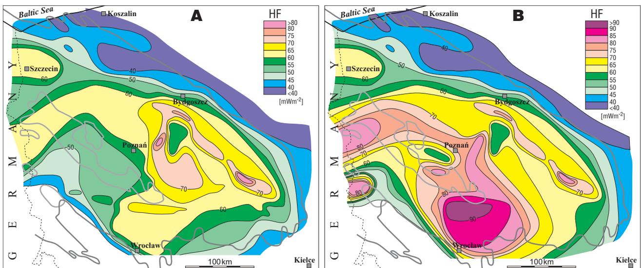
**Fig. 8.** Map of average heat flow values in the area of Polish Permian Basin obtained from the computer simulations: A — from the Cretaceous to the Recent present time; B — the Late Permian to the Late Jurassic period
