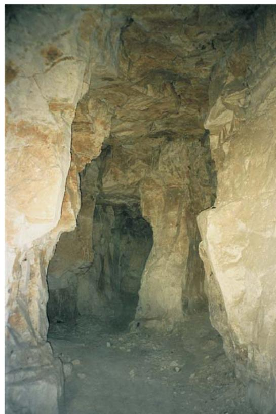
Fig. 9. The chamber exploitation of opokas in the Bochothnica quarry. Photo by B. Bąk
