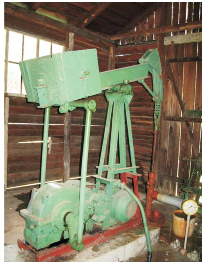
Fig. 10. An old pump abstracting saline water from a borehole in Rabka-Zdrój. Photo by L. Rajchel
