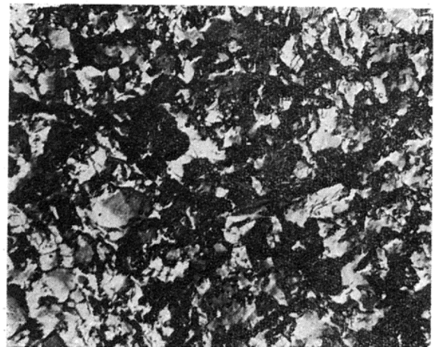
Figs 6—7. Direct replica of broken surface of decalcified gáize sample from Lechówka; fragment of rough-knobby surface; X 5000.
