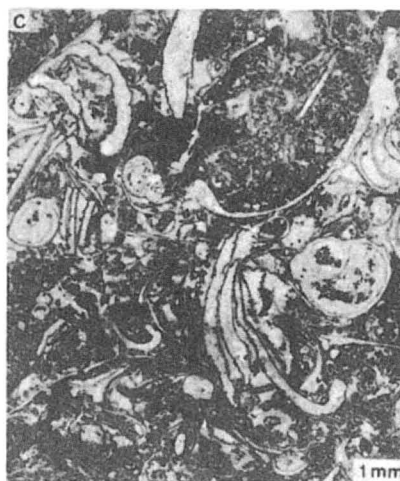
Fig. 4. A — Laminated mudstone, with grainy interlayers (at the bottom). Dopiewo 2, depth 2960.0 m. B — Bioclast-peloid packstone-grainstone. Gaj 2, depth 3122.2 m. C — Recrystallized bioclast grainstone. Swadzim 1, depth 3074.8 m
