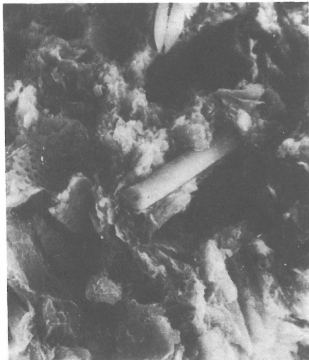
Fig. 2. SEM micrographs of horizontal surfaces (a and b) of the Chmielnik clays taken at different magnifications.
