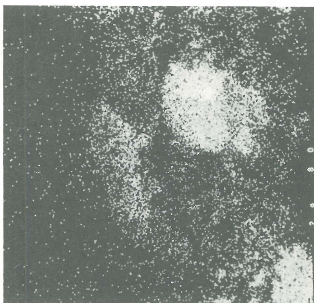
Fig. 7. Microstructure (SEM) and qualitative analysis of distribution of elements (microprobe studies) in rust-coloured quartz, ×480.
