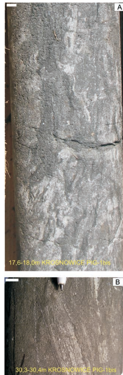
Fig. 5. Core samples from borehole Krosnowice PIG-1bis. A – core section from a depth of 17.6–18.0 m: dark mudstone and white, medium-grained sandstone showing nearly vertical, irregular bedding planes; B – core section from a depth of 30.3–30.4 m: dark, fine-grained sandstone with visible sub-vertically disposed sedimentary lamination. Scale bar is 1 cm long in all photographs.
