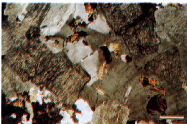
Fig. 4. The Niegoslawice granite. K-feldspar contains inclusions of plagioclase, biotite and pale green hornblende. Note late brittle shear and faulting. Scale bar 1 mm.
