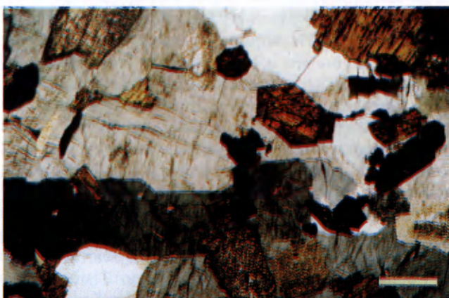
Fig. 5. The Gościszowice granite. Plagioclase, hornblende and biotite form inclusions in K-feldspar. Scale bar 1 mm.
