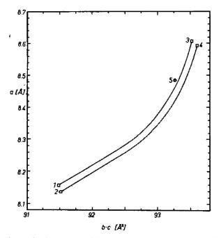
Fig. 5. The dependence of the *a* parameter on the *b*·*c* values of the alkali feldspars according to Bernotat (Kroll, Ribbe 1983). The feldspars with the strained lattice parameters have their projection points outside the area bordered by the lines 1-3 and 2-4. 1 – analbite; 2 – low albite; 3 – high sanidine; 4 – low microcline; 5 – sanidine of Wielisławka Hill
