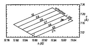
Fig. 7. The relation between the ordering degree expressed by the  $2t_1$  value and the *b* and *c* parameters of the alkali feldspars, after Kroll and Ribbe (1983). 1 - analbite; 2 - high sanidine; 3 - sanidine from Wielisławka Hill
