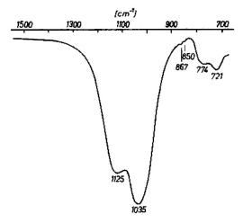
Fig. 6. The infrared absorption spectrum of the Wielisławka sanidine
