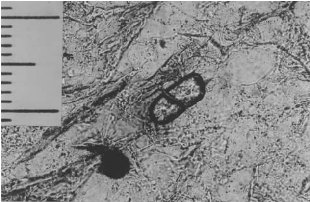
Fig. 8. Subrounded zircon grain split into two parts by a fracture transversal to its elongation. The fracture is filled with synkinematic chlorite; one polarizer, small unit on scale = 0.01 mm.
