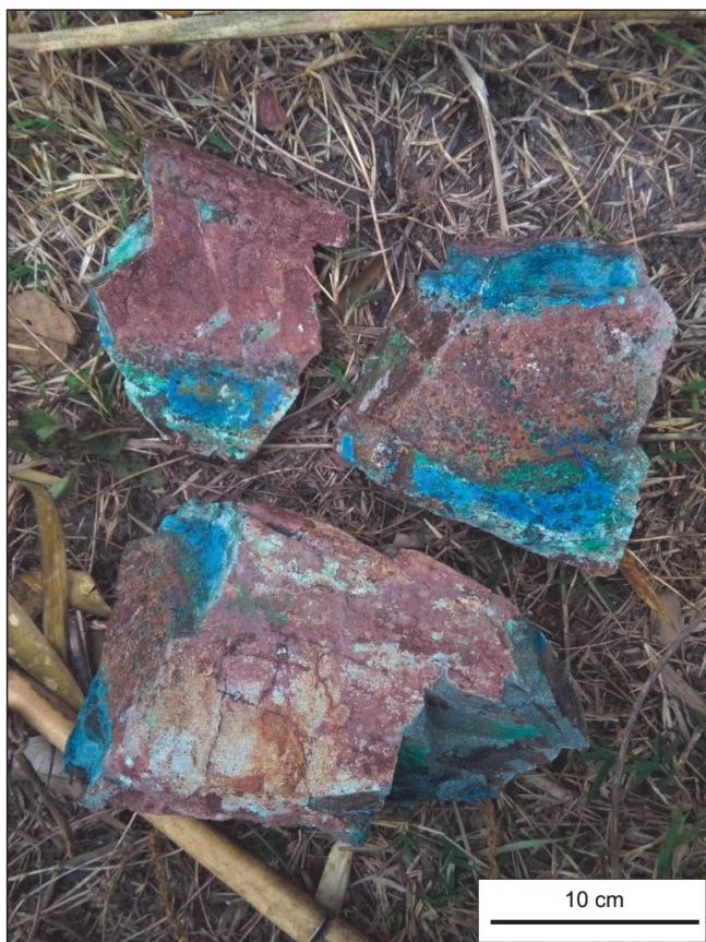
Fig. 3. Rock samples taken from an abandoned mine, with visible copper-bearing mineralization. Photo by K. Zglinicki, 2018
