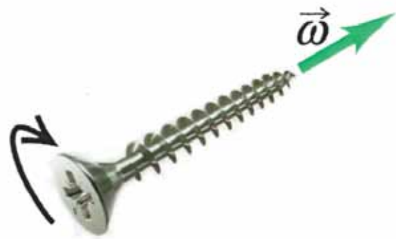
Fig. 2. Dextrorotatory-screw rule determining the sense of vector of angular velocity
