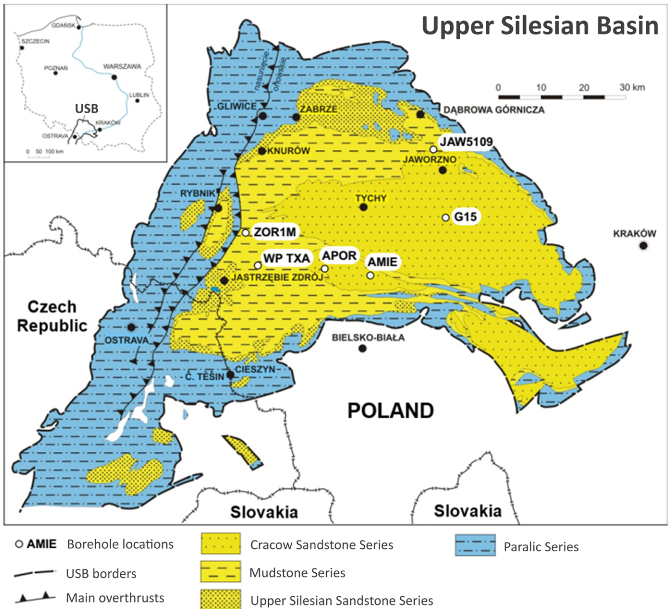
Fig. 1. A simplified geological map of the Upper Silesian Basin (USB) after Jureczka et al. (1995), with the locations of the investigated boreholes.
