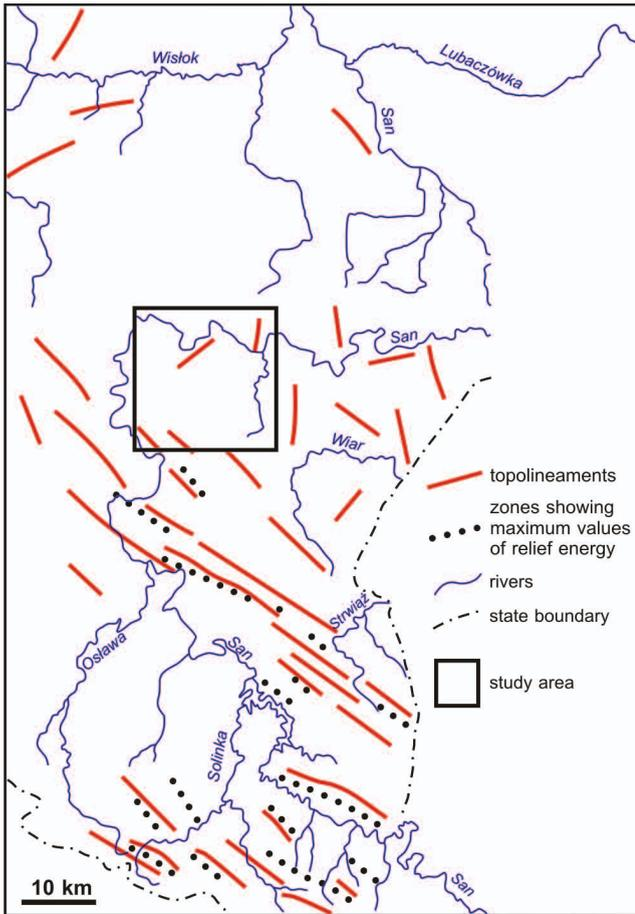
**Fig. 10.** Principal topolineaments and zones of maximum relief energy in the eastern portion of the Polish Carpathians interpreted from dense-contour relief energy map, showing location of the study area (modified from Zuchiewicz, 2000)
