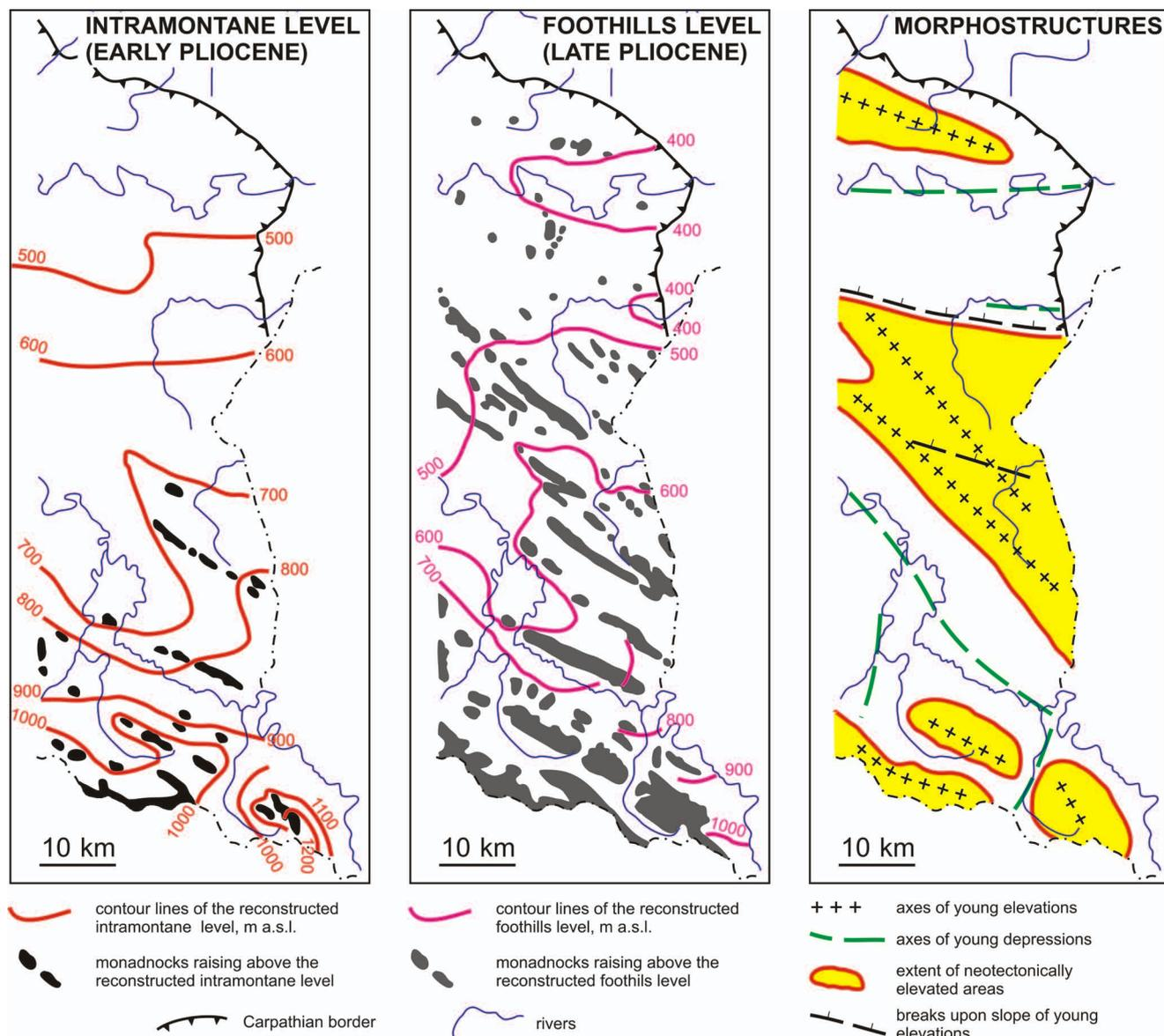
**Fig. 12.** A reconstruction of topography and neotectonic structures during formation of the Pliocene planation surfaces in the eastern segment of the Polish Carpathians, as proposed by (Henkiel, 1977); see also Zuchiewicz (2000)
