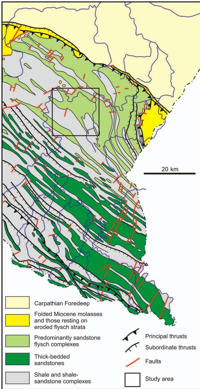
**Fig. 3.** Map of rock resistance in the eastern portion of the Polish Carpathians (based on Borysławski *et al.*, 1980; Gucik *et al.*, 1980; Żytko *et al.*, 1989; modified). See Fig. 2 for location
