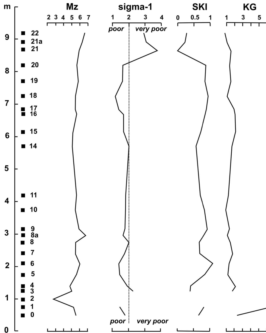
Fig. 5. Grain-size characteristics of the Janowice section, showing differentiation of basic Fold and Ward's (1957) parameters: Mz – graphic mean diameter ( \phi ), sigma-1 – graphic standard deviation, SKI – graphic skewness, KG – graphic kurtosis
