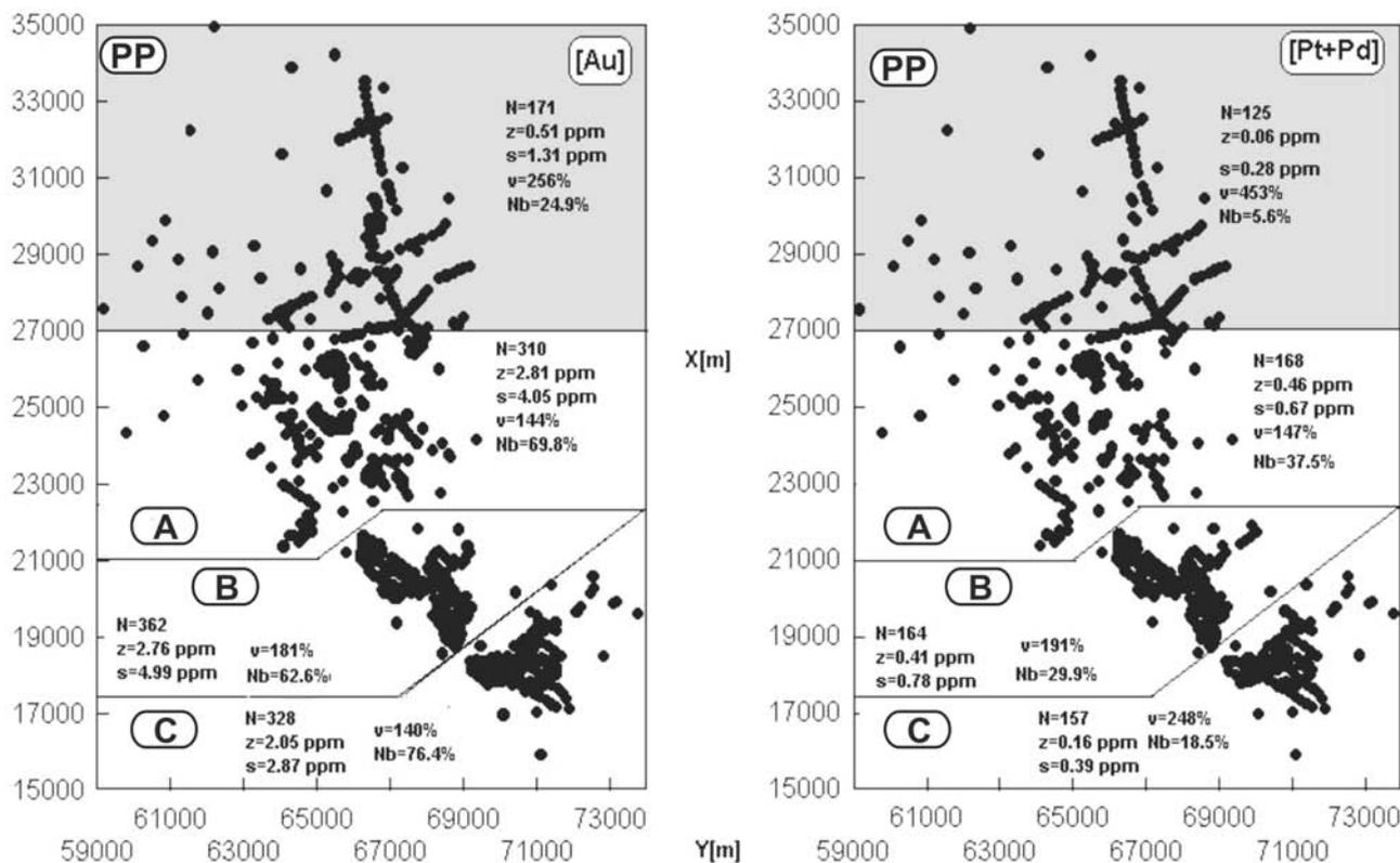
**Fig. 96.** Samples location for assaying of the gold content [Au] and the platinum and palladium content [Pt+Pd] in the Cu – Ag ore deposit Polkowice-Sieroszowice. PP – sub-economic part of deposit, PB – economic part of the deposit, A, B, C – areas of exploration. N – Number of samples,  $\bar{z}$  – arithmetic mean, s – standard deviation, v – coefficient of variation, Nb – proportion of samples with grade above 0.5 ppm
