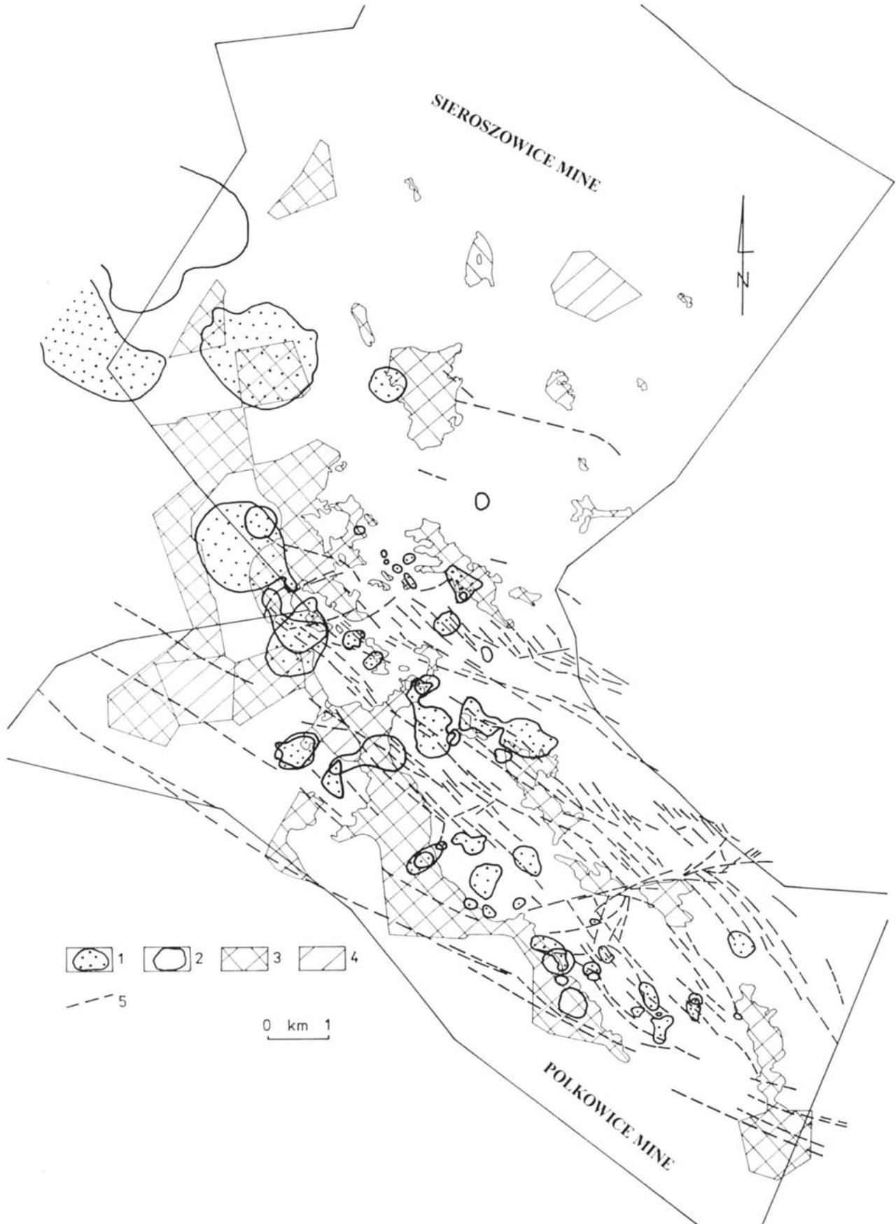
**Fig. 100.** Superposition map of rich gold and PGM fields on the back ground of basic tectonics. 1 – area with minimum content of Au = 2 ppm, 2 – area with minimum content of Pt + Pd = 1 ppm, 3 – area without economic copper deposit, 4 – area with sub-economic copper deposit, 5 – documented faults
