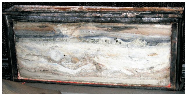
Fig. 9. One of the “mini-aquarium” tanks, in which Dżułyński conducted many of his experiments to produce deformational structures, now displayed in the Museum of the Institute of Geological Sciences of the Jagiellonian University, Kraków. The tank is approximately 65 cm long and 15 cm wide. (Photo by G. Kelling)
