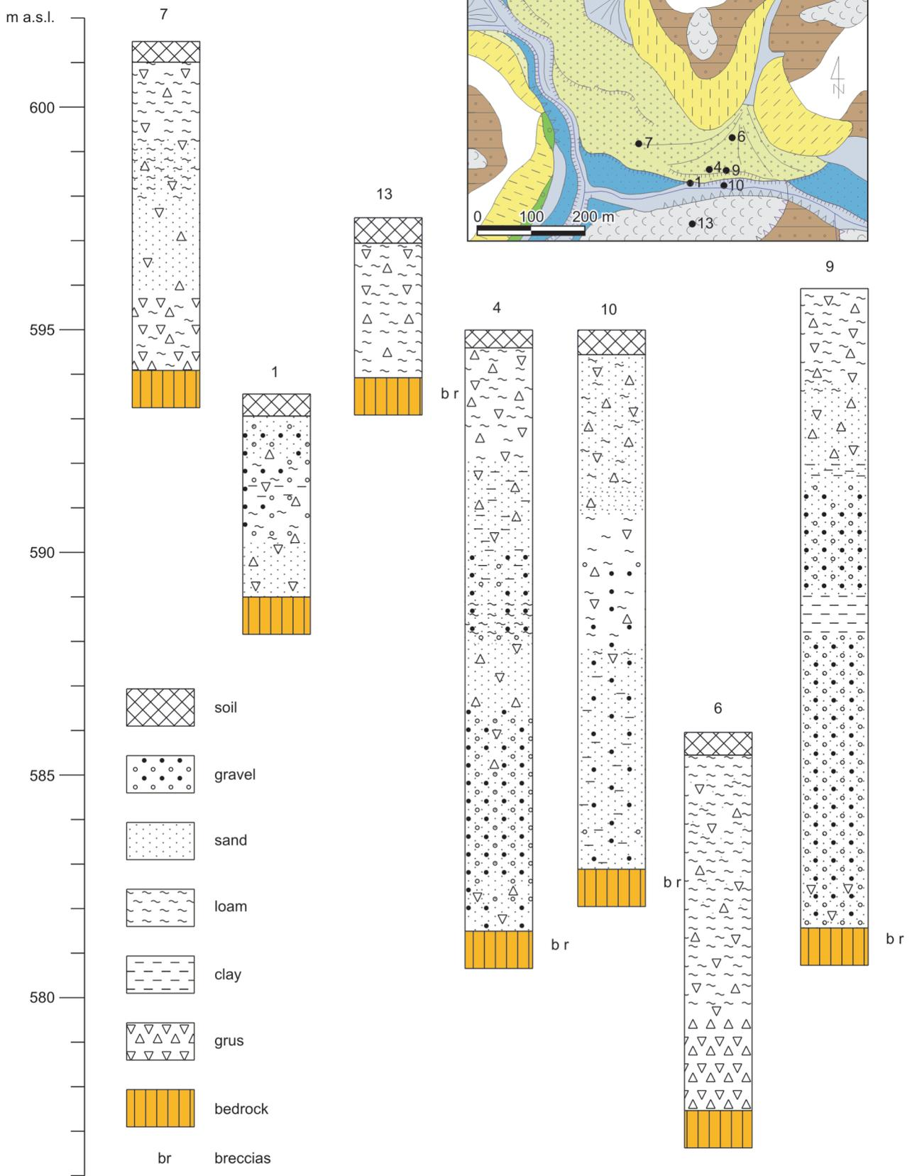
**Fig. 11.** Lithology of Quaternary sediments exemplified by terraces and alluvial fans at the confluence of the Palenica and Kryniczanka rivers at Krynica Spa (borehole data based on Fistek & Szarszewska, 1987). See Figs 2 and 8 for location
