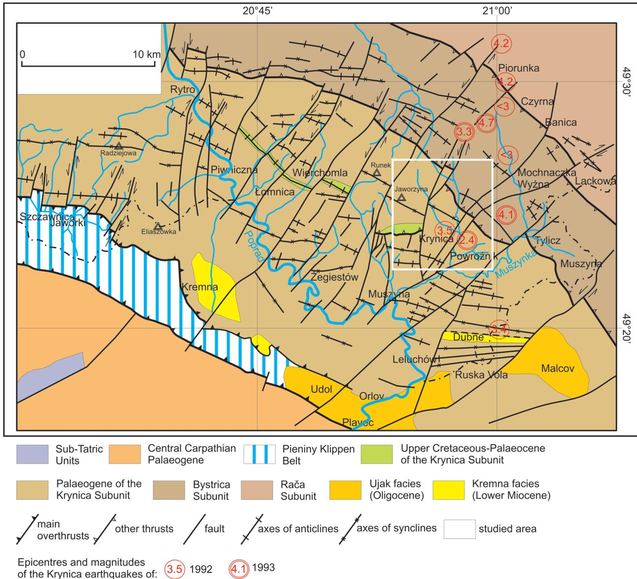
**Fig. 7.** Tectonic sketch map of the SE part of the Beskid Sądecki Range and NW part of the Lubovnianska Pohorkatina Range (based on sheets of the Detailed Geological Map of Poland, 1: 50,000; as well as Nemčok, 1990 and Oszczytko *et al.*, 2005)
