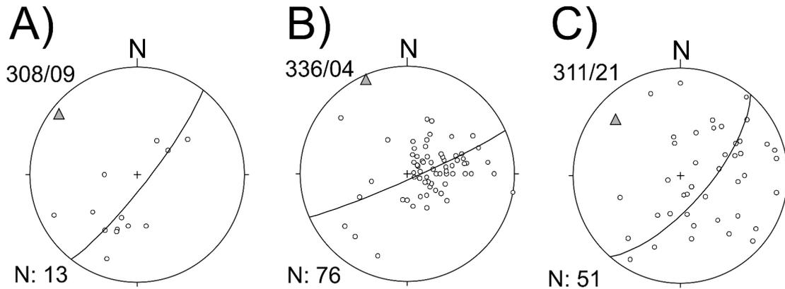
**Fig. 5.** Bedding attitude in the Krynica area.  $\pi$ -diagrams and orientation of map-scale folds in: **A** – Bystrica subunit (NW part of the Kryniczanka drainage basin); Krynica subunit: **B** – NW part of the Kryniczanka drainage basin, **C** – SE part of the Kryniczanka drainage basin. Lower hemisphere plot
