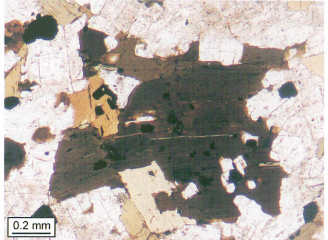
Fig. 11. Red-brown biotite in granodiorite (transition zone), borehole DB-5, depth 1370.0 m. Plane-polarized light
