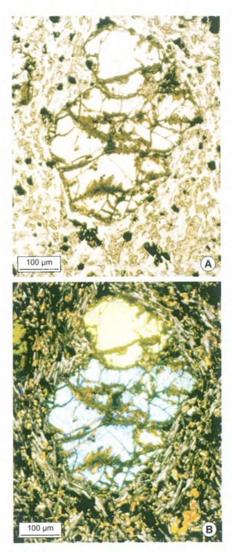
Fig. 15. Photomicrograph of cracks in olivine phenocryst filled with serpentine-group minerals. Olivine basalt intrusion at Męcinka, site BP-33: A – one nicol; B – crossed nicols
