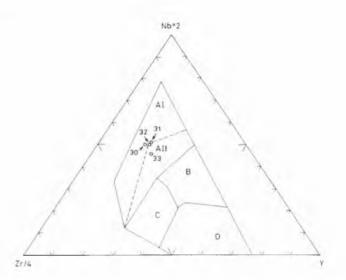
Fig. 10. Plot of basaltic rocks (samples BP-30-33) in the Zr-Nb-Y discrimination diagramme of Meschede (1986). Al – within-plate alkaline basalts; All – within-plate alkaline basalts and within-plate tholeiites; B – E-type MORB; C – within-plate tholeiites and volcanic-arc basalts; D – N-MORB and volcanic-arc basalts
