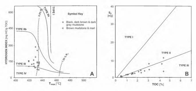
**Fig. 28.** Type of kerogen determined by Rock-Eval pyrolysis in the fine-grained rocks in which TOC exceeds 0.5%. **A.** Type of kerogen indicated by the relation between hydrogen index and the temperature of maximum hydrocarbon evolution ( $T_{max}$ ). **B.** Type of kerogen indicated by the relation between total organic carbon content (TOC, in %) and the amount of hydrocarbons evolved from the thermal alteration of the kerogen (S; in milligrams, normalized to sample weight)
