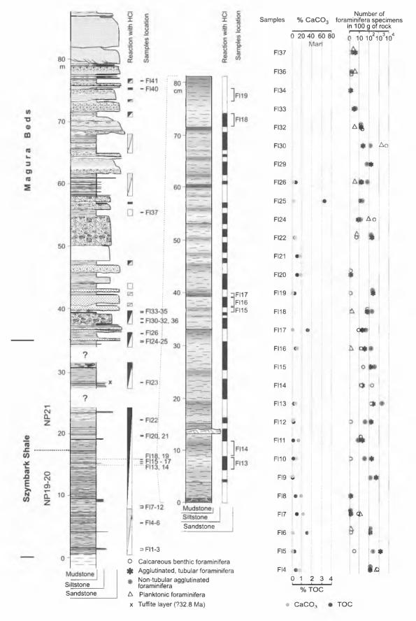
**Fig. 26.** Graphic log of the Szymbark Shale and the lower part of Magura Beds outcropped in the bed of Kłopotnica stream in Folusz (see Fig. 5A for section location), reaction with diluted HCl, TOC, CaCO<sub>3</sub> and foraminifera contents in the fine-grained sediments. Calcareous nannoplankton zones cf. Tab. 1 and Oszczypko-Clowes (2000, 2001). For other symbols, see Fig. 9
