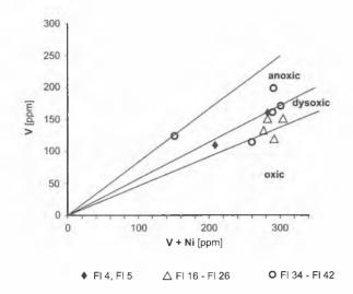
**Fig. 29.** Vanadium/vanadium + nickel plot of the fine grainedsediments from the Szymbark Shale (samples Fl4, 5 – lower part; samples Fl16-Fl26 – upper part) and the lower part of Magura Beds (samples Fl34-Fl42) in the Folusz section. The fields of oxygenation regime are after Lewan (1984)
