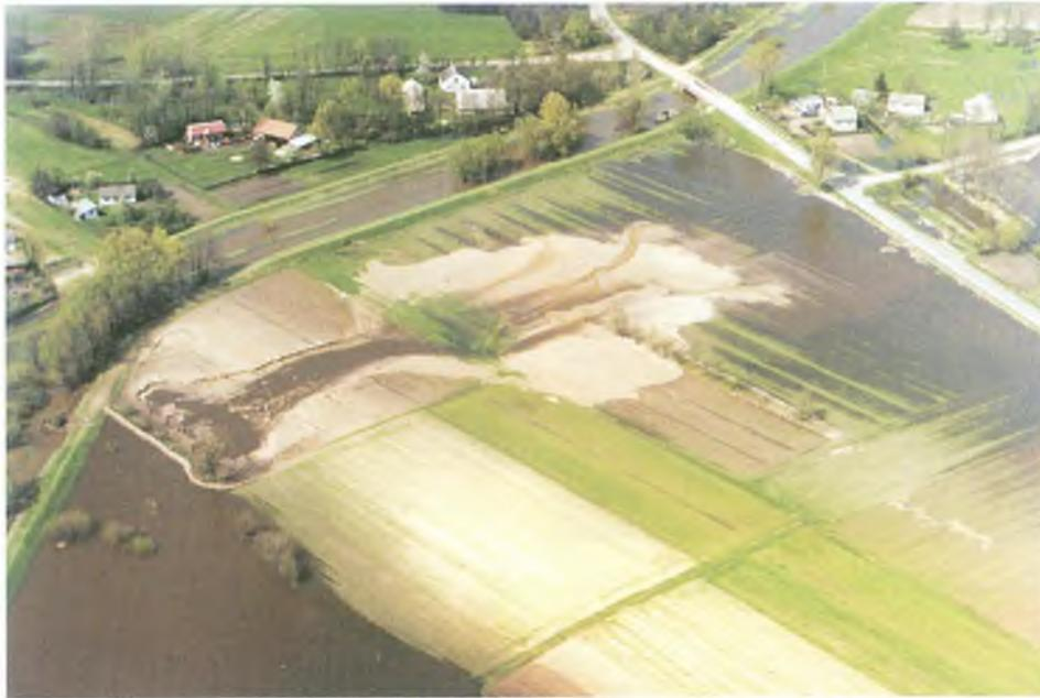
Fig. 2. The Upust Stream, embankments, dune, crevasse and crevasse splay (oblique air photo)
