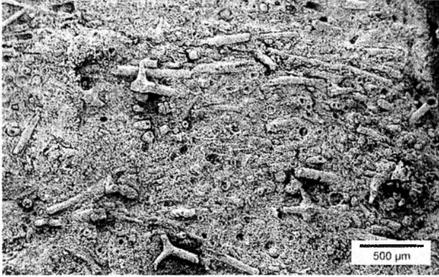
Fig. 9. A distinctive accumulation of siliceous sponge spicules. Parallel arrangement of spicules is visible. SEM image of HF etched surface; Huciański Klin crest
