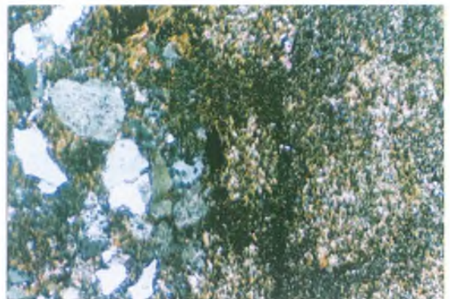
Fig. 3. Sharp boundary between metasandstones and fine-grained cordierite hornfels. Borehole DB-5, depth 905.3 m. Crossed polars
