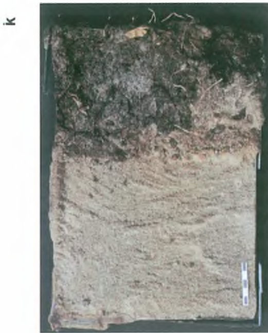
Fig. 11. Channel sand from the bottom of a main channel, peat clasts in the upper part. Vertical sample taken using wedge-shaped sampler, impregnated with epoxy resin; scale in cm
