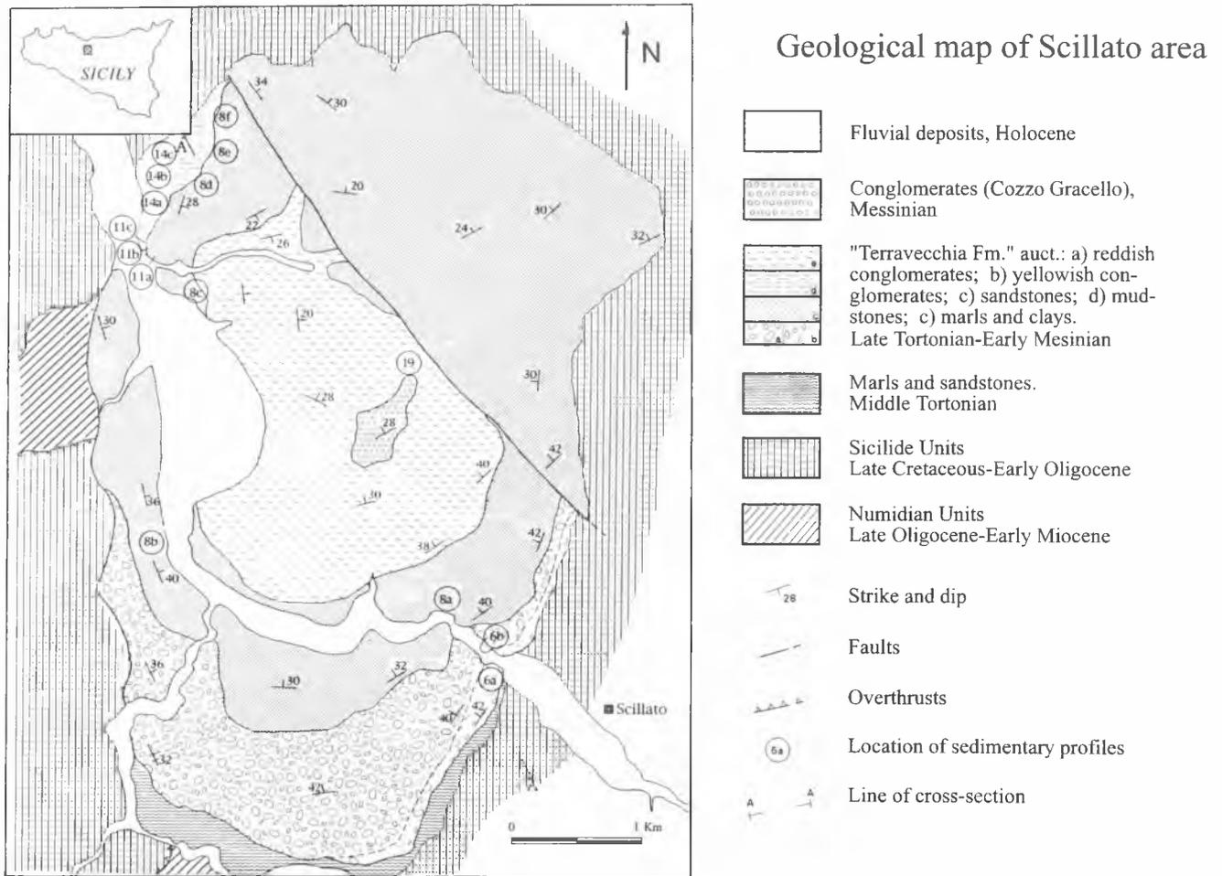
Fig. 2. Geological map of the Scillato Basin. Numbers in circle refer to numbers of figures with litho-stratigraphic sections
