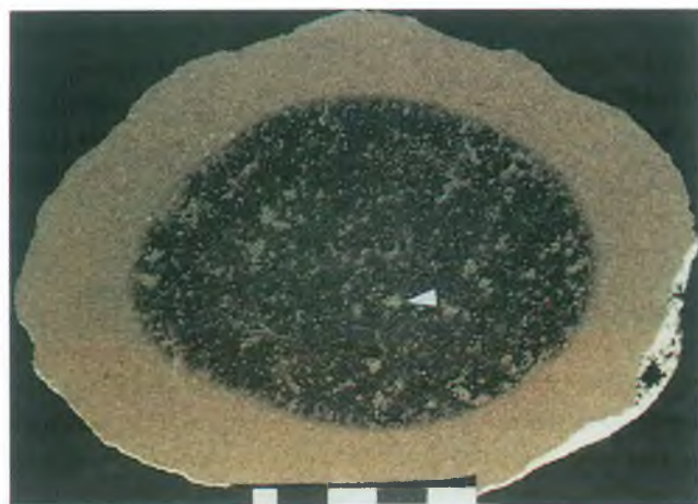
Fig. 4. Polished slab of an exotic organodetritic Lithothamnium limestone of calcarenitic type. Irregular outer surface is visible along with central cherty core which reflects the shape of the surface and contain equally spaced enclaves of unsilicified rock (arrowed). Site 4 (Kosztowa); bar scale in centimetres
