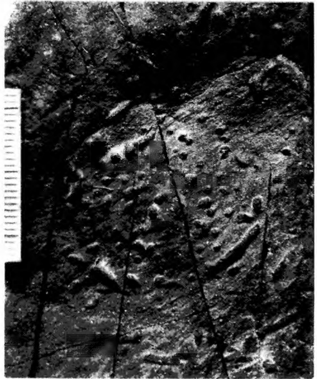
Fig. 108. Form B. Sole of a turbiditic sandstone bed. UJ TF 1797, Zawoja-Końskie (part of label lost). Scale in mm
