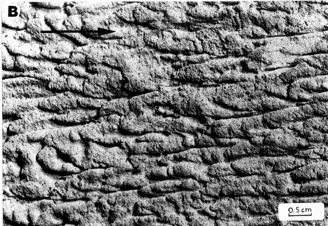
Plate 34 (A) Moulds of l-ridges and furrows with incipient scales. Oligocene Krosno beds, Rudawka Rymanowska. (B) Moulds of l-ridges and furrows with incipient scales. Base of artificial turbidite (after Dżułyński, 1965)
