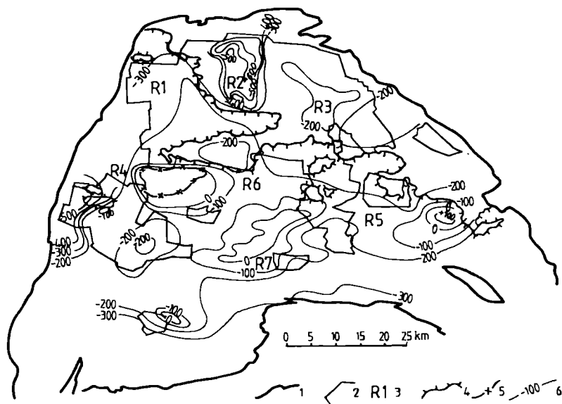
Fig. 2 Hydrochemical regions and depth of occurrence of brines ( \text{TDS} > 35 \text{ g/dm}^3 ). 1 – depth contour; 2 – extension of the isolating series of the Tertiary deposits; 3 – extension of the salt deposits; 4 – extension of the coalfields; 5 – hydrogeological regions; 6 – hydrochemical regions
