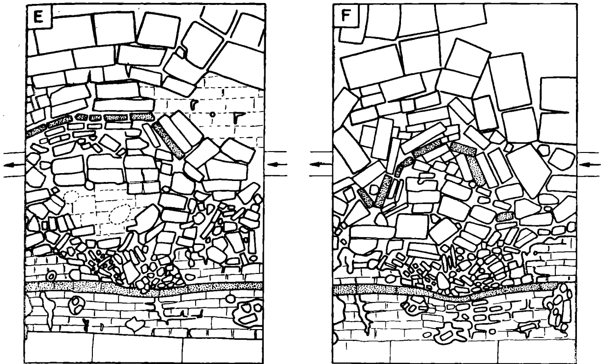
Fig. 2. Experimental effects of dissolution in horizontal and fractured layers under constant phreatic conditions. Flow of water from right to left (arrow). „A”...„F” successive stages of dissolution and deformation. Progressive (down-current) and retrogressive (up-current) development of longitudinal caves is initiated from input and discharge sides of the main tank. Note transverse solution caverns fixed along fractures and intersections of fractures. Transverse caverns are produced by water diverted from main flow towards observer. „F” shows final collapse breccia with solutionally obscured lower boundary. Detached and broken fragments of upper stippled layer indicate extent of vertical displacement of fragments. Note solutional rounding of fragments close to lower boundary of breccia
