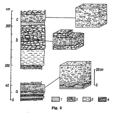
Intraformational conglomerates (layers a, b, c) in the Wellenkalk at Wincentów 1 micritic limestones, 2 crumpled limestones, 3 marly limestones, 4 marls
