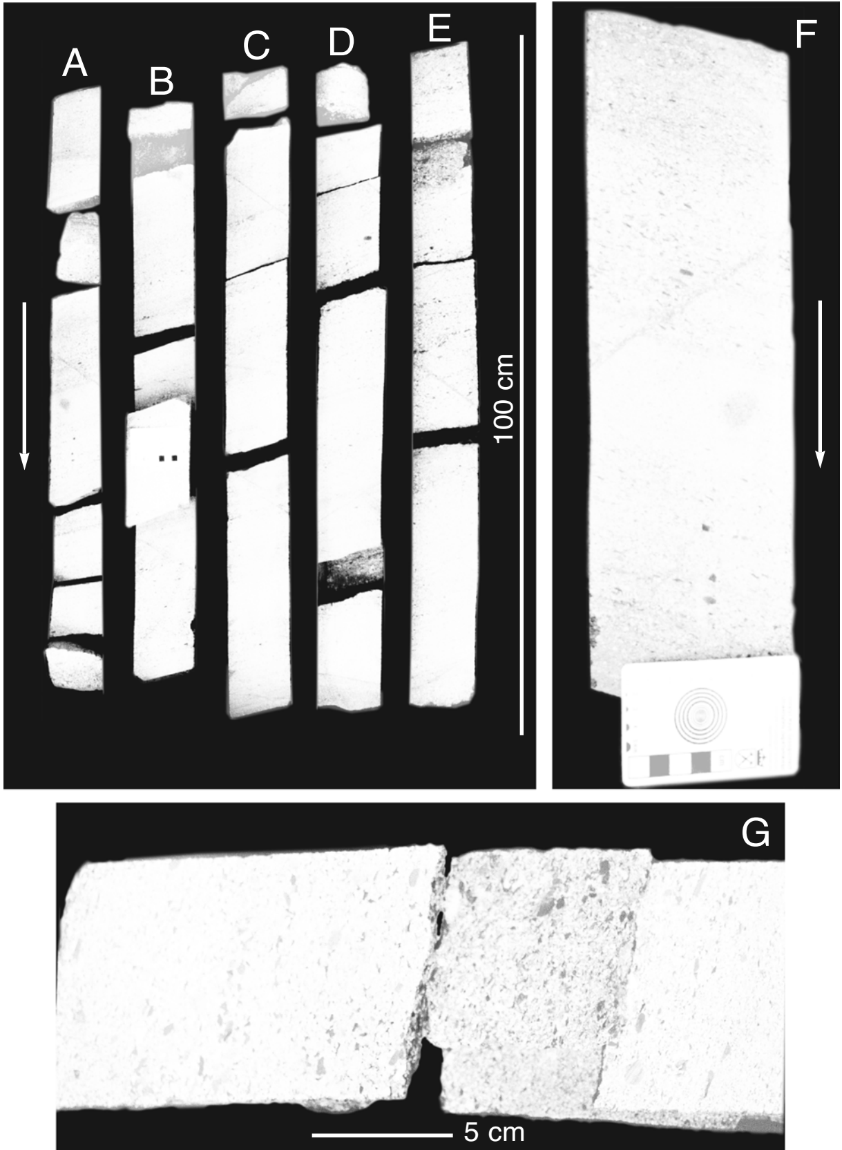
Fig. 4. Andrychów 6 borehole – core interval 2135-2143 m. Granule conglomerates and coarse- to very coarse-grained sandstones of the Dębowiec Conglomerate. A – box (S I), B – box (S II), C – box (S III), D – box (S IV), E – box (S V), F – Thin-bedded granule conglomerate and planar laminated, graded-bedded, very coarse to coarse-grained sandstone, cut through low-angle, early diagenetic inverse fault (detail from box (S I), G – Small scale imbrication of the granule conglomerate, detail from box (S V)
