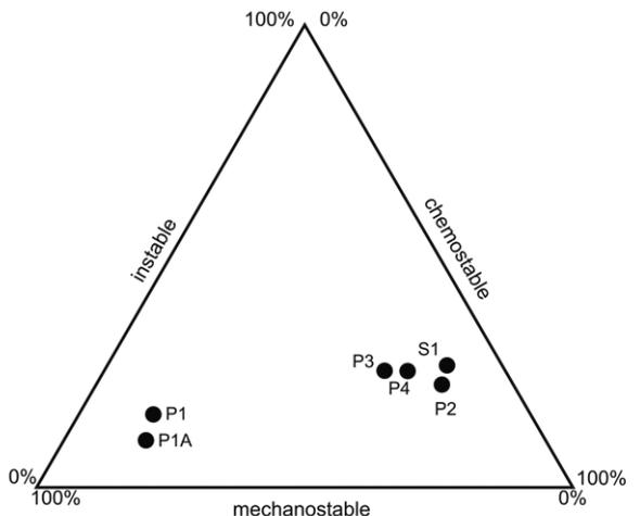
Text-fig. 10. Relationship between instable, chemostable and mechanostable heavy minerals in the studied samples, classification diagram after Burkhardt (1978)
