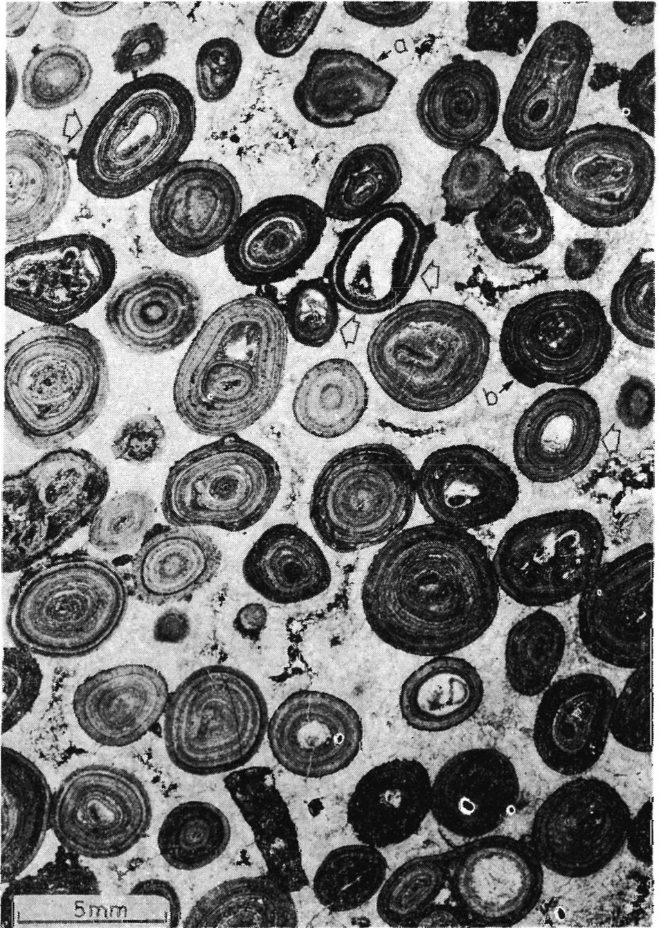
Loosely packed and well sorted oolite, some ooids of which are complex, and some reveal the half-moon effect (arrowed); abraded ooids ( \alpha , \beta ) are also indicated. Locality Wurmbrandegga
