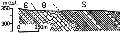
Fig. 18 Large drag folds in the Ordovician and Silurian deposits exposed along the stream running down from Mt. Jeleniowska, east of Jeleniów
