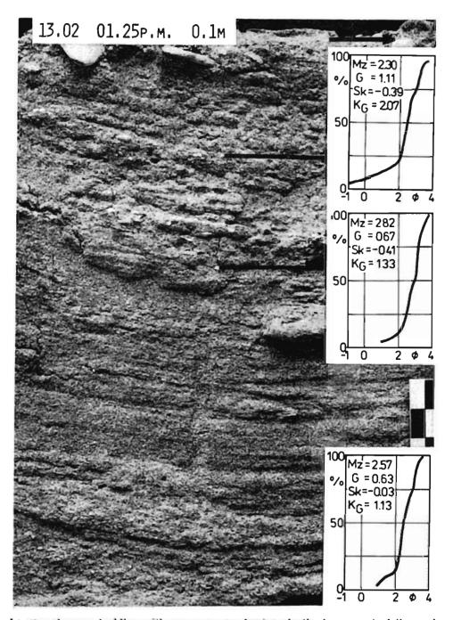
Large-scale cross bedding with concave cross laminae in the lower part of the sand ridge slope; a polychaete burrow reaches the upper boundary of a finer sediment
