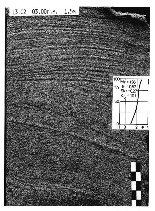
Two large-scale sets with cross bedding; the lower set corresponds to the landward slope of the first sand ridge, and the upper one to an almost flat surface of the landward slope of the successive sand ridge
