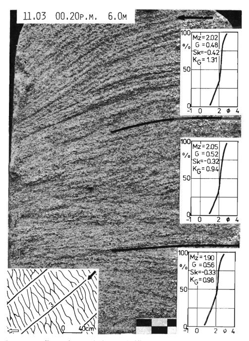
Large- or medium-scale megaripple cross bedding with small and varying inclination and with increasing inclination of convex cross laminae in the upper cross set, corresponding to the rising slope of the megaripple; sample yields no traces of cross bedding connected with the ripples recorded in the pattern scheme
