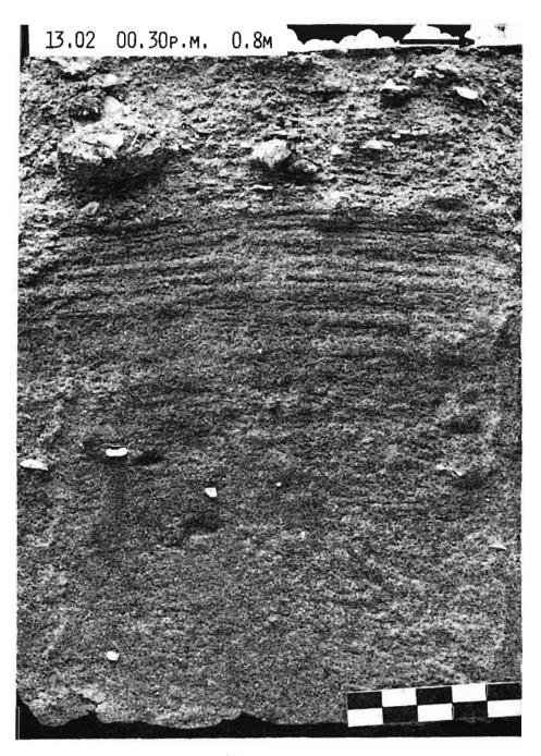
Horizontal bedding in the fine-grained sediment, heavily bioturbated (bottom), and coarse sediment (top) with pebbles and shell fragments oriented
