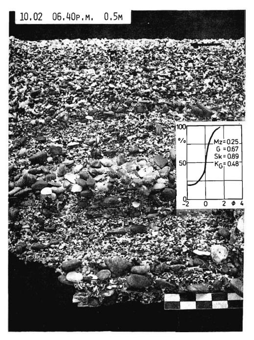
Nearly horizontal or large-scale cross bedding in gravel sediment of the lower part of the beach slope; orientation of pebbles and shell fragments is well visible
