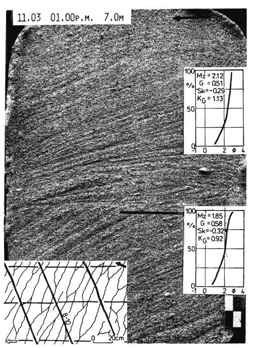
Two cross sets of large-scale megaripple cross bedding separated by an erosional boundary and showing increasing inclination of cross laminae in the upper set, corresponding to the rising slope of the megaripple
