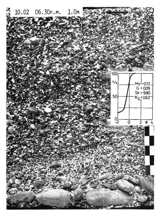
Slightly inclined bedding (flat pebbles are oriented) in the sample collected from the base of the beach slope
