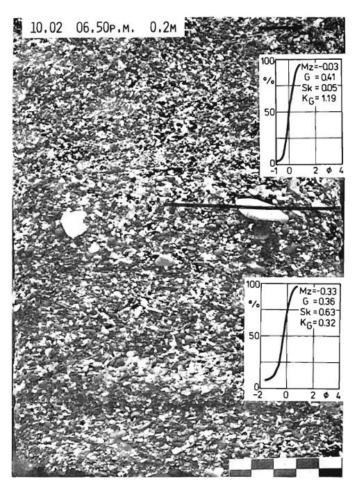
Vague, nearly horizontal or large-scale cross bedding in coarse sediment of the upper part of the low-inclined beach bar
