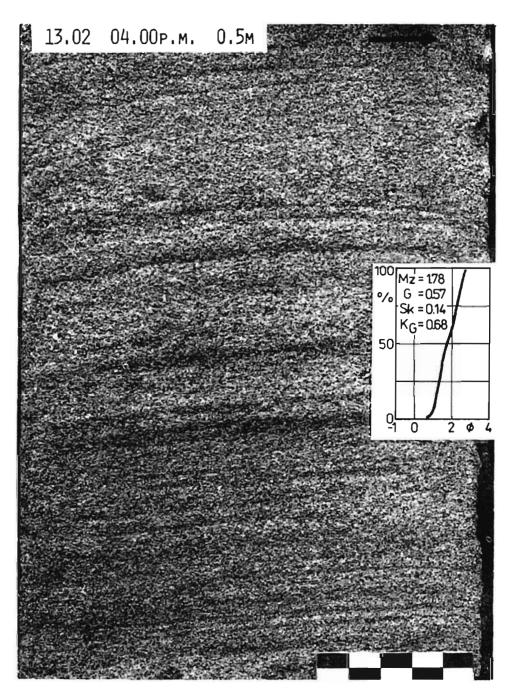
Low-angle cross bedding in a sample collected from the central part of the beach slope
