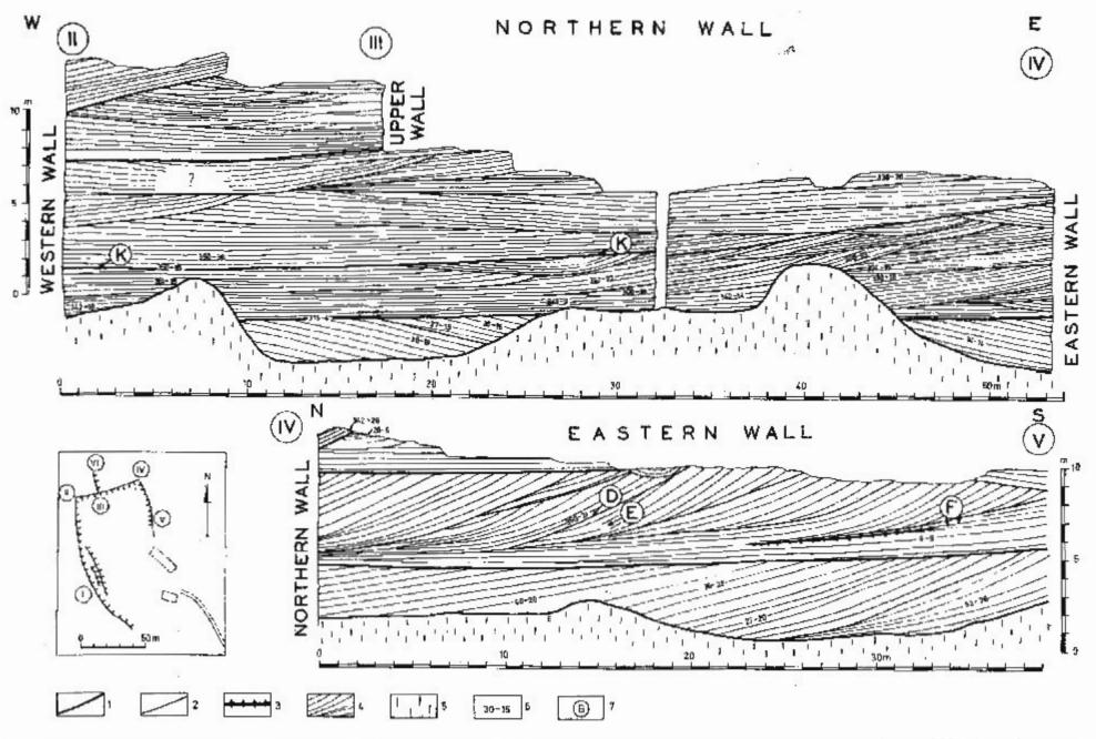
1 — main bounding surface; 2 — additional bounding surface; 3 -- layer with mud-cracks; 4 — selected strata; 5 — rubble; 6 — direction of true dip and angle of true dip (both values in degrees);
