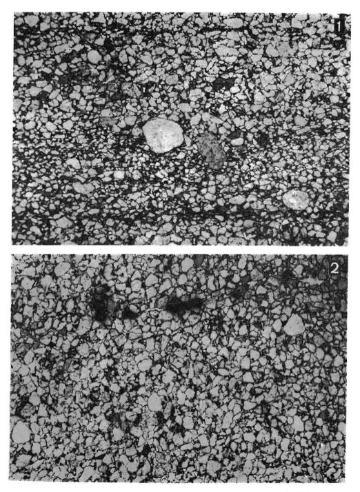
1 — Isolated larger grains in laminated sandstone of association B (thin section 49),  $\times$  12 2 — Structureless sandstone filling erosional channel (thin section 62),  $\times$  12
