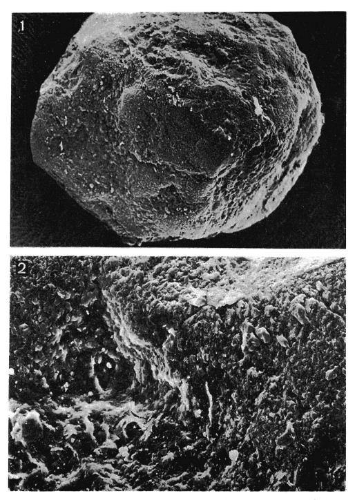
Scanning electron micrographs: 1 — Quartz grain,  $\times$  325; 2 — Upturned plates modified by solution and precipitation,  $\times$  1950
