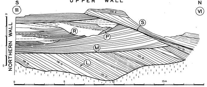
L — deformations of cross-laminae in form of overthrusts (see Pl. 8, Fig. 2); M — subhorizontal main bounding surface (cf. Text-fig. 5 and Pl. 6, Figs 1 & 2); P - slided and rotated block at bank of erosional channel; R — deformations at bank of erosional channel (see Pl. 14, Fig. 1)
