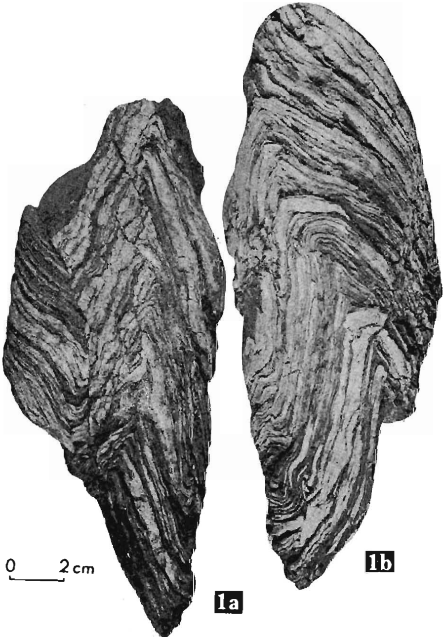
1a—b — Tectonic disturbances in siltstone formed probably in the near fault zone. Pionki 4, sample 28, 1938.4—1934.0 m
