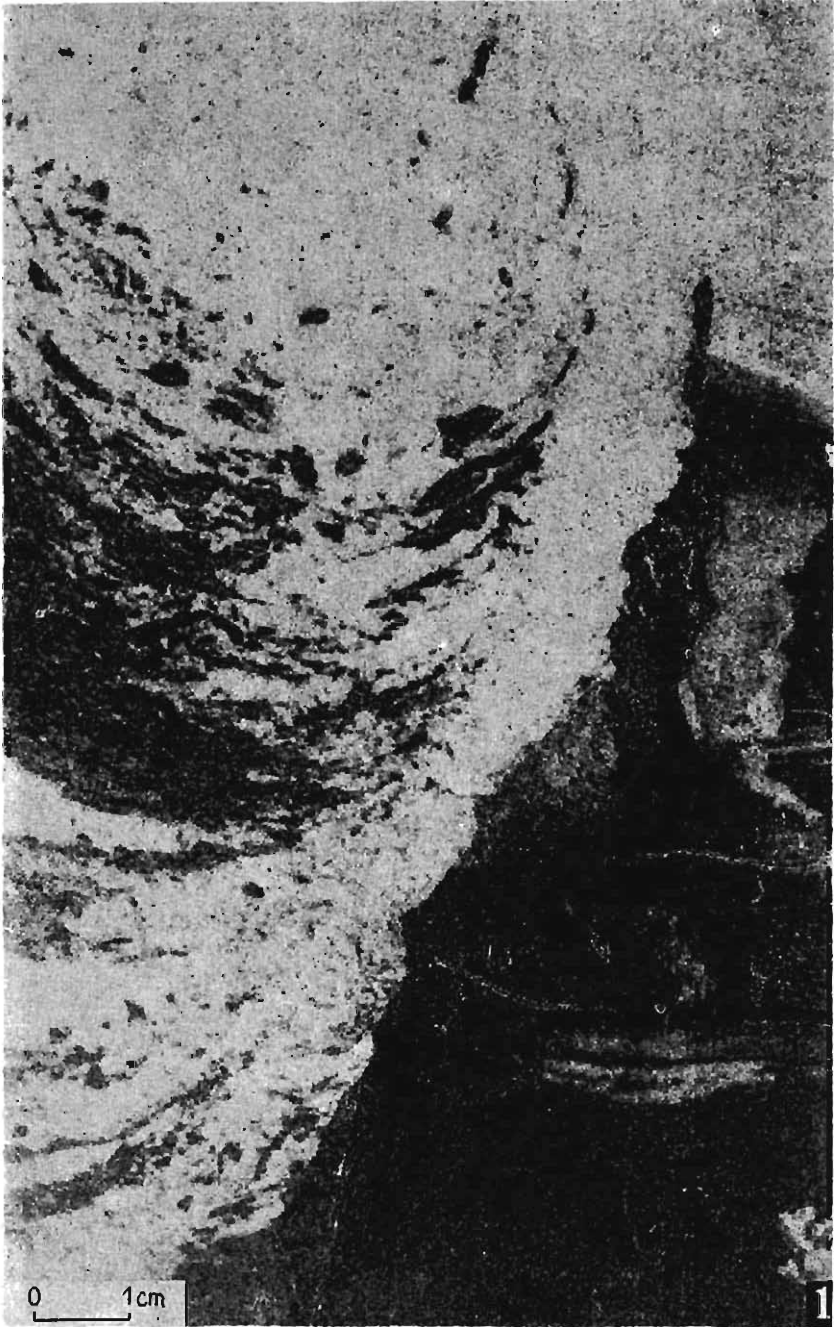
1 — Load structures at the boundary of two rock types: underlying dark siltstone and overlying light sandstone. At left interbeds of dark siltstone bent bottomward. Primarily possibly horizontal. Pionki 4, sample 17, 2438.3—2432.3 m
