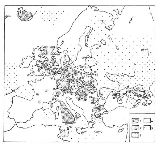
Fig. 5. Map of heat flow in Poland included to the map of heat flow in Europe (after Majorowicz 1977 a)  $1 - Q \ge 2.0; 2 - 1.6 - 2; 3 - 1.4 - 1.6; 4 - 1.0 - 1.4; 5 - Q < 1.0$  (in heat flow units  $10^{-6}$  cal/cm<sup>2</sup>s)
