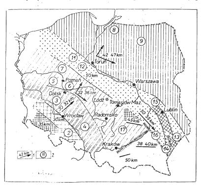
Fig. 8. Scheme of geotectonic division of the Polish area from studies of the Earth's crust and upper mantle by deep seismic sounding methods (after Guterch 1977)
