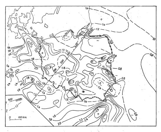
Fig. 4. Map of heat flow in Poland and in adjacent areas (after Majorowicz 1977) I - position of the international deep seismic profile VII; 2 - isolines of heat flow in 10<sup>-6</sup> cal/cm<sup>2</sup>. s
