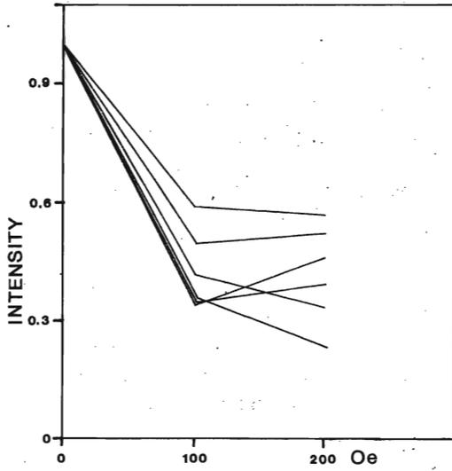
Fig. 2. Intensity of residual magnetism in samples No. 1 to No. 6 from Nasiłów depicted as intensity versus demagnetization field
