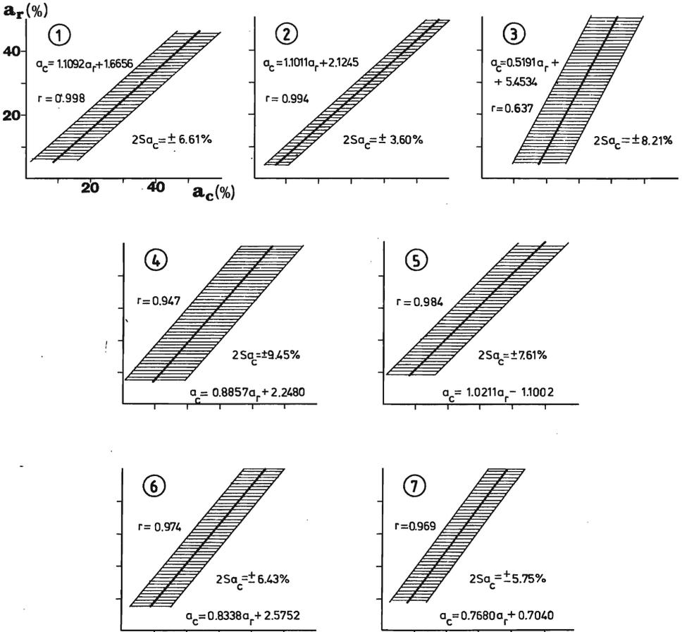
Fig. 9. Statistic relationship between true grains of a given size class in a sample ( $a_r$ ) and sectioned true grains ( $a_c$ ) of the same class (identified by the color of apparent grains); other explanations as in Text-fig. 8, with modification of regression equation: here is of  $a_c = ma_r + n$  type
