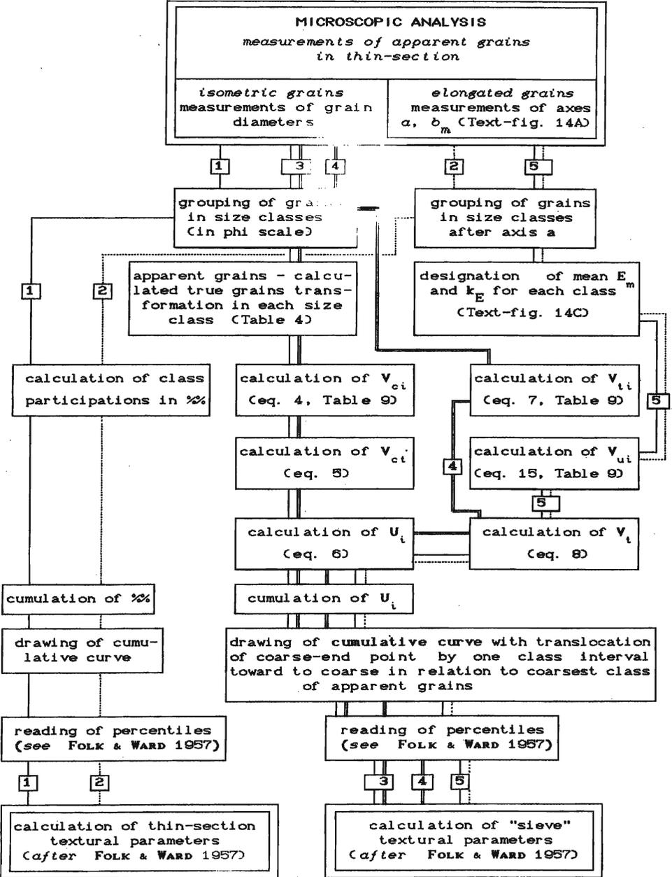
Determination of thin-section parameters: for isometric apparent grains — path 1, for elongated apparent grains — path 2
