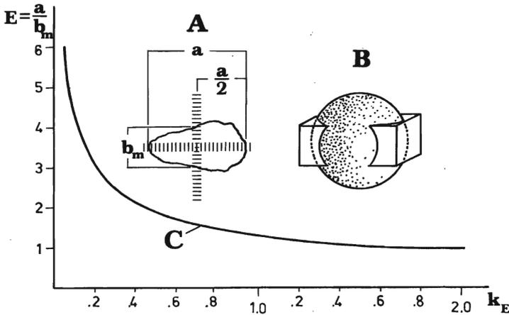
Fig. 14. Interrelationship between an elongated apparent grain, a calculated grain, and a spheroidal grain
