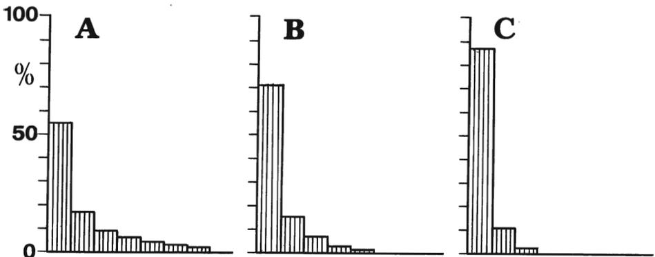
Fig. 11. Histograms of theoretical distributions of apparent grains from the same sized true grains, for different analytical intervals: A — 0.25, B — 0.50, C — 1.00 phi; the single stud represents one size class
