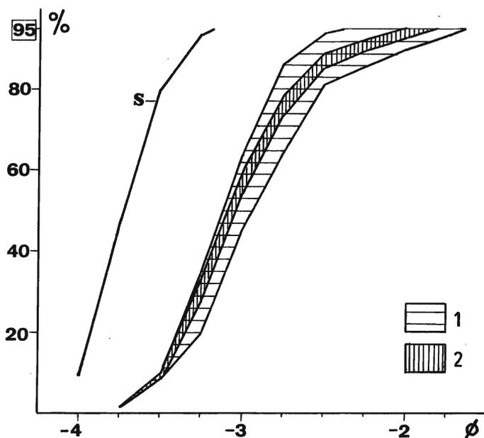
Fig. 2. Cumulative curves of grain size distributions of the pilot-sample *A*
